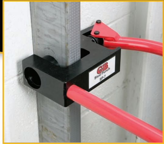
Punches 1 1 / 32 " holes for 1/2" to 1" conduit or pipe in aluminum and mild steel studs
