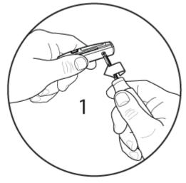
1. Use a Phillips head screwdriver to loosen the screw. Leave the screw engaged. (Figure 1)
