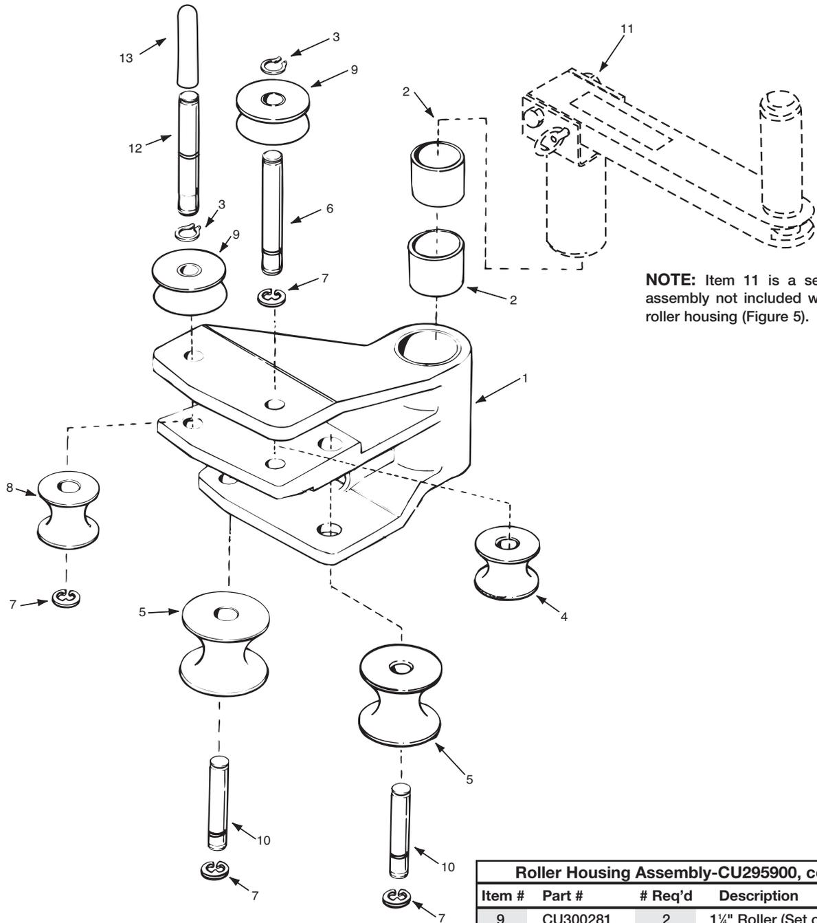
**NOTE:** Item 11 is a separate assembly not included with the roller housing (Figure 5).
