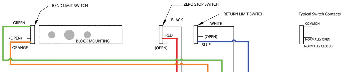
2. Verify that the black wire goes to the pin on the limit switch that is separate from the other two, and that the red wire is connected to the middle pin.
