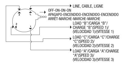
NOTE: This is a push-in / stab-type style switch. In order to insert the wires into the switch, you must have 18 AWG solid wire. If you do not have solid wire, you most solder the 18 AWG stranded wire together. You must be careful not to push the flap down to hard while inserting the wire as to much force will ruin the switch.
