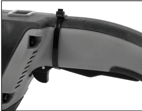
Figure 16. A cable tie or strap may be needed to keep trigger squeezed
