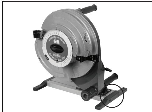
Figure 22. Remove Screws to Remove Feet
