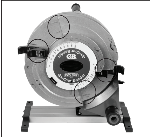
Figure 2. Conduit Size and Type Indication Markings
