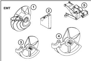
**BEMT-52** – For bending 1/2" thru 2" EMT (Thinwall) *Includes the following six items:*
