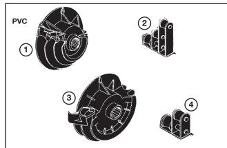
**BPVC-52** – For bending 1/2" thru 2" 40 mil PVC coated RIGID *Includes the following five items:*
