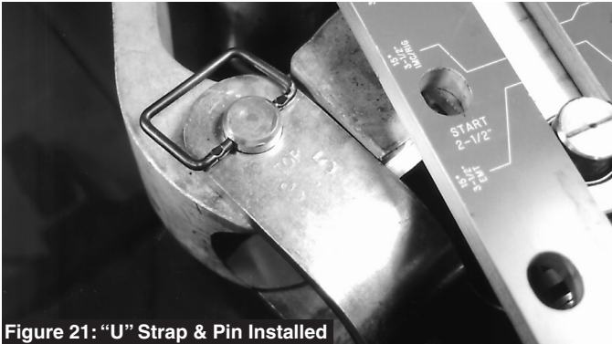
Figure 21: “U” Strap & Pin Installed
