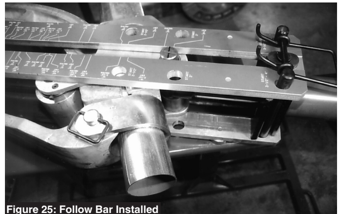
Figure 25: Follow Bar Installed
