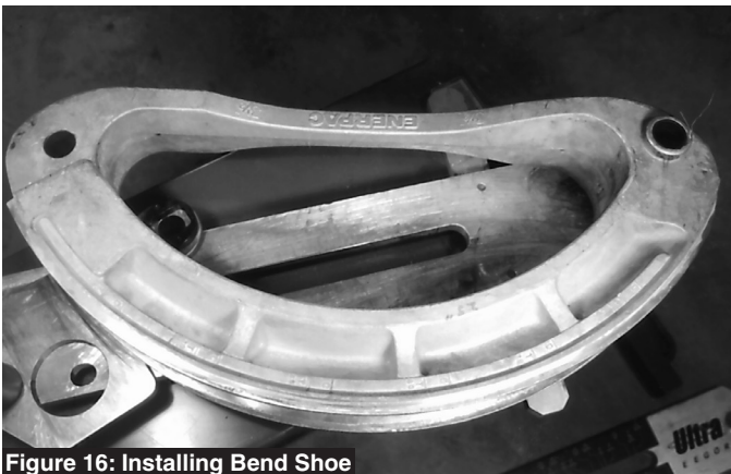
Figure 16: Installing Bend Shoe
