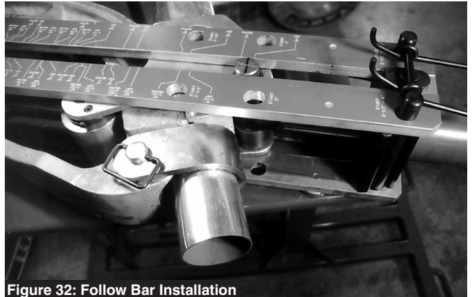
Figure 32: Follow Bar Installation
