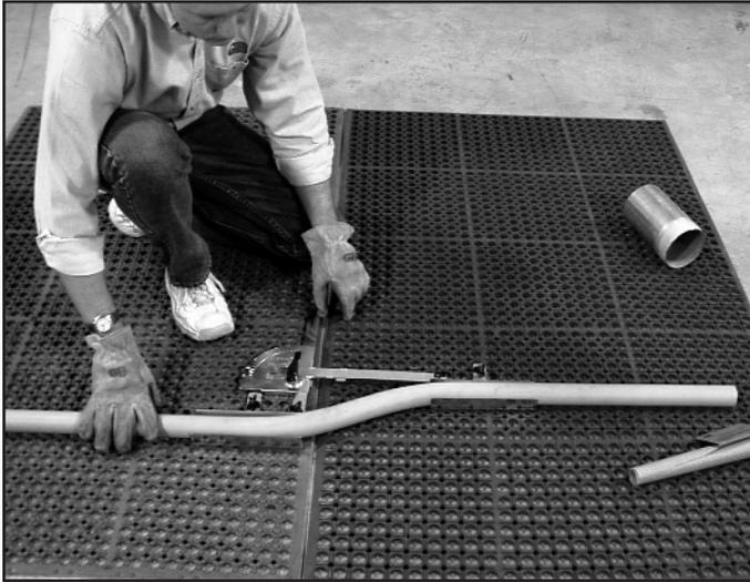
5. Hold the pipe in the bent position until the bend is set and the pipe has cooled enough to handle without gloves. Wipe pipe with a wet rag to set the bend and cool the pipe.
