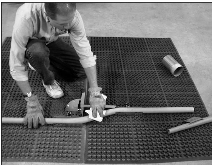
**Note:** Remove kinks or ripples prior to cooling pipe. After the pipe is cool the bent area cannot be heated again and reformed.
