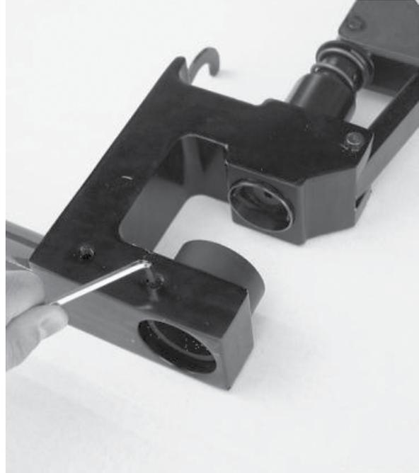
2) To remove die loosen the hex bolt closest to the die located on C-frame.
