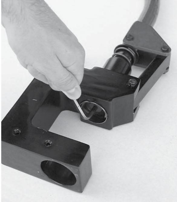
1) To remove punch from SP-7 unscrew hex bolt at center of punch using a #5 hex wrench.
